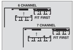
(5) With the track in place on top of the brackets rotate each of the locking clamps until they touch the back of the track, starting with the centre bracket. It may be necessary to gently tap the clamps with a light hammer to lock them into place.
