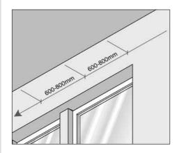
(2) Draw a straight line along the top of the wall where the track is to go and mark on this the position of the brackets. Each end bracket should be no more than 10cm from the ends of the track and each subsequent bracket should be spaced equally apart at 60-80cm intervals.
