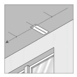
2 A template is supplied which shows the correct drill positions for your track. The FRONT LINE on the template refers to the position of the front of the track facing into the room. Draw a straight line along the ceiling marking the FRONT LINE of the track, ensuring clearance of doorhandles, sills etc is maintained along the full length.
