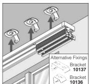
(6) Offer the track up to the brackets. Start at the centre and rotate locking clamps until they touch the back of the track. Depending on your fixing you may need to gently tap the clamps with a light hammer to lock into place. Move along the track until all the clamps are locked.
