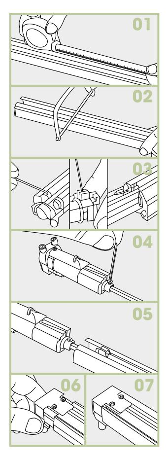
Using a T10 torx key tighten up both screws on the top side of the headrail as well as the single screw on the bridge.
