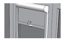
To lock the blind into position, rock the hande backwards.
