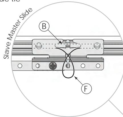
NOTE: Cord should be tensioned so that the Tension Pulley is slightly extended.
