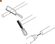
If cutting down, when you are certain your measurements are correct, mark the pole and cut. Wrap masking tape around the pole to avoid damage. File any sharp edges and drill a small hole in the centre of the pole.
