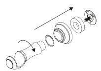
Assemble the brackets onto the back plates and secure by turning the bracket body clockwise until it is tight. Ensure that the cup is upright on completion of tightening.
