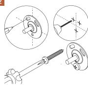
On your horizontal line mark the bracket positions using the back plate as a guide.
