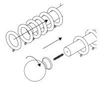
Slide the rings on to the pole. Secure the finial on to the end of the pole by tightening it in place.
