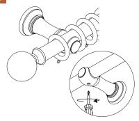
Place the pole on the brackets with the last ring on each side between the finial and end bracket. Finish by tightening the screws to ensure your pole is secure.
