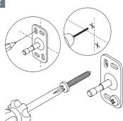
On your horizontal line mark the bracket positions using the back plate as a guide.
