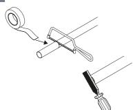
If cutting down, when you are certain your measurements are correct, mark the pole and cut. Wrap masking tape around the pole to avoid damage. File any sharp edges.
