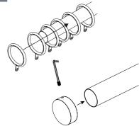
Slide the rings on to the pole. Secure the finial on to the end of the pole by tightening the grub screw.
