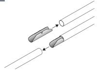
If joining 2 poles together, use the joining piece provided ensuring that it fits **INSIDE** the poles. The poles must be joined in the centre and supported by the centre bracket.
