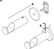
Assemble the brackets, push onto the back plates and secure by tightening the grub screw. 4
