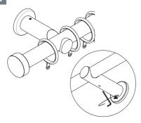
Place the pole on the brackets with the last ring on each side between the finial and end bracket. Finish by tightening the grub screws to ensure your pole is secure.
