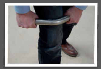
**3.** You can bend by hand to the angle you need, checking as you go. Alternatively use an angle measurer/bevel/protractor to find the angle, then bend accordingly.
