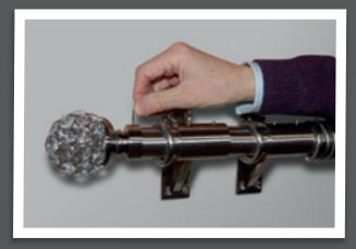
**7.** Finally, ensure that all the poles are level and then use the allen key to tighten all the brackets. Fit the finials and fit the magnetic cover plates to the centre bracket.
