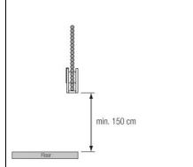
This retaining device should be installed at the maximum distance possible from the control mechanism to prevent the looped pull cord(s) becoming slack.
